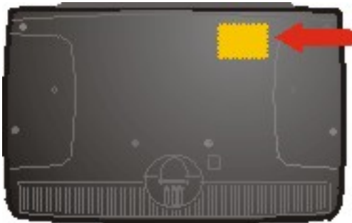
Figure 1 CDRH / IEC 825 Caution Label Location – MX3X, Back
