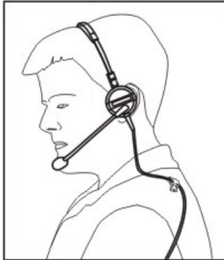
The headset consists of an earpiece, a microphone, a clothing clip and a cable. The headset attaches to the audio cable end of the voice cable which attaches to the MX9.
