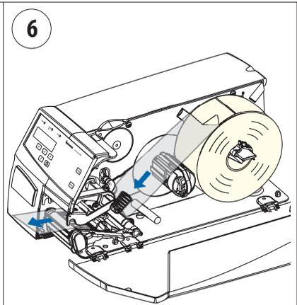
Remove labels from the first 50 cm (20 inches) of the liner. Route the liner through the print mechanism and push it inwards.
