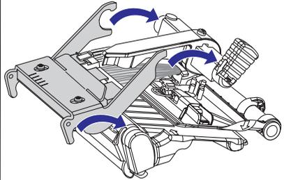
Put back the printhead in reverse order and check that the printhead cables run freely.
