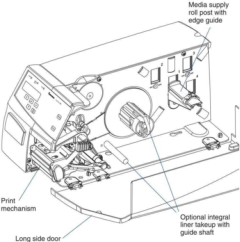
The EasyCoder PF2i uses a media supply roll post that can be fitted in three different positions inside the media compartment. The position depends on the type of side door (long or short) and whether or not the printer is fitted with an integral liner takeup. Alternatively, an external media supply (for example a box of fan-folded tickets) behind the printer can be used. A rotating media supply hub is also available as an option, see Chapter 8, “Options.”
