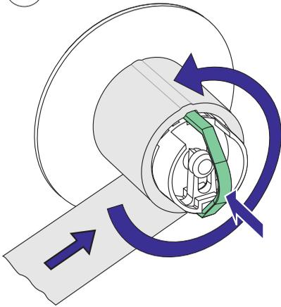
Press the handle to expand the takeup hub and secure the liner. Then rotate the hub counterclockwise until the liner becomes tight.
