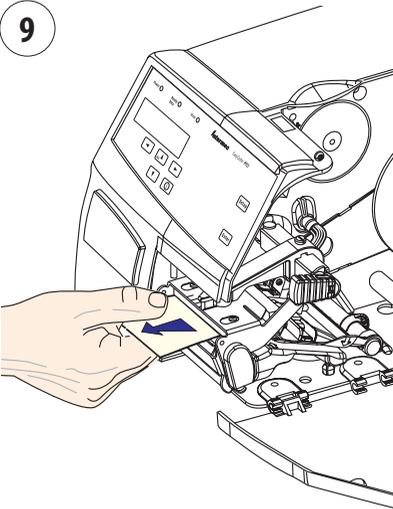
Pull out the cleaning card. If necessary, repeat the process with a fresh cleaning card.
