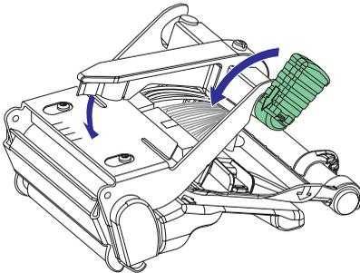
Turn the printhead lift lever counter-clockwise so the magnet engages the printhead bracket.
