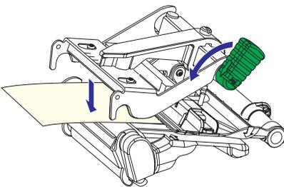
Turn the printhead lift lever counter-clockwise to engage the printhead.
