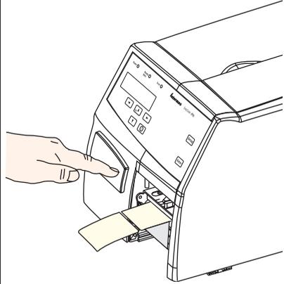
*Press the Feed/Pause button to advance the media and adjust the media feed.*
