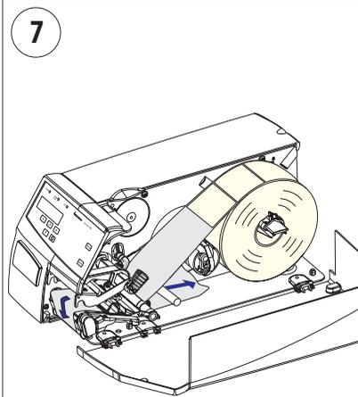
Route the liner around the tear bar and the liner drive roller and back under the print mechanism and guide shaft.
