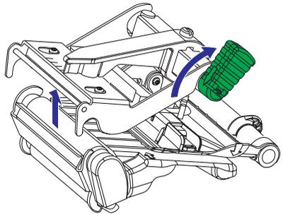
Turn the printhead lift lever clockwise to raise the printhead.
