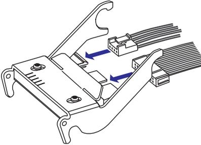
Connect the two cables to the replacement printhead.
