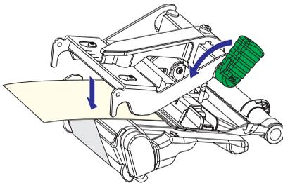
Turn the printhead lift lever counterclockwise to engage the printhead.
