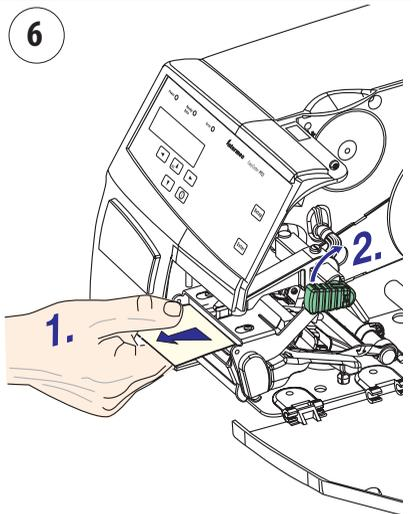
Pull out the cleaning card (1) and raise the printhead (2).
