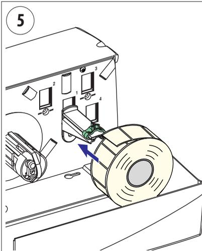
Fit a new roll of labels on the supply post and adjust the edge guide so the label roll becomes flush with the center section.
