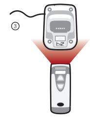
Scan the Batch Mode Transfer All Data in Memory\* configuration barcode to transfer data to the host device.
