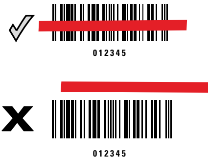
Figure 3-3 Scanning Orientation with Aiming Line
