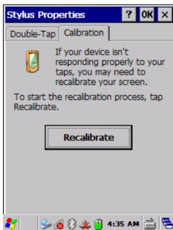
2. Tap **Align Screen** to open the **Calibration** screen shown in the figure below.
