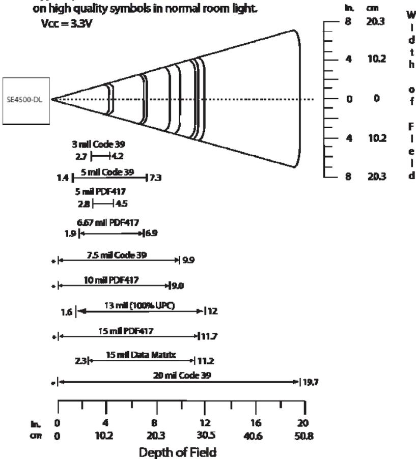
\* Minimum distance determined by symbol length and scan angle.
