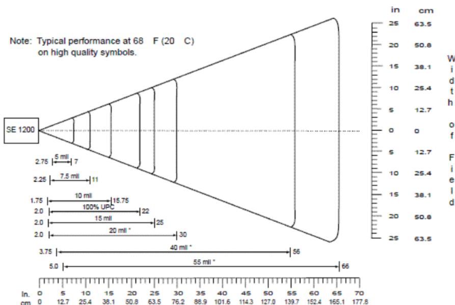
\*Minimum distance determined by symbol length and scan angle
