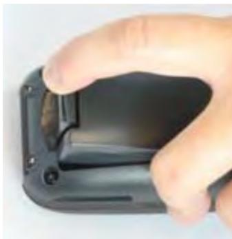
3. Open the Micro SD card slot by pulling up the locking plate:
