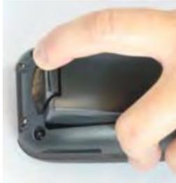
3. Install the new battery pack, first insert the top end, then the latch bottom as indicated in the following figure.
