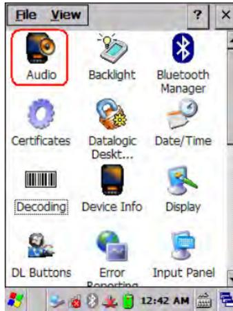
The Audio applet allows to set the recording volumes of the main microphone and of the headset microphone. Also, it allows to set the headset volume when the user is listening to an audio file.
