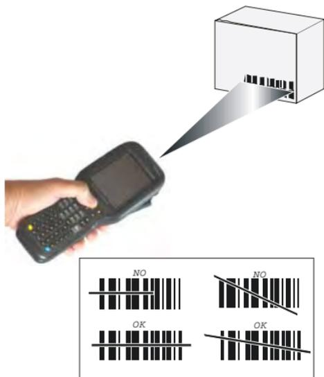
The XLR engine includes a pointer mode that projects a highly visible scan line at longer ranges to make it easier to accurately target bar codes. The user simply holds the trigger down until the aimer is on the appropriate code. Releasing the trigger then initiates the bar code scan.
