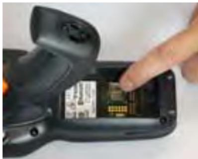
4. Insert the Micro SD card with the written part upward. Lock the card into place by pushing the cardholder down:
