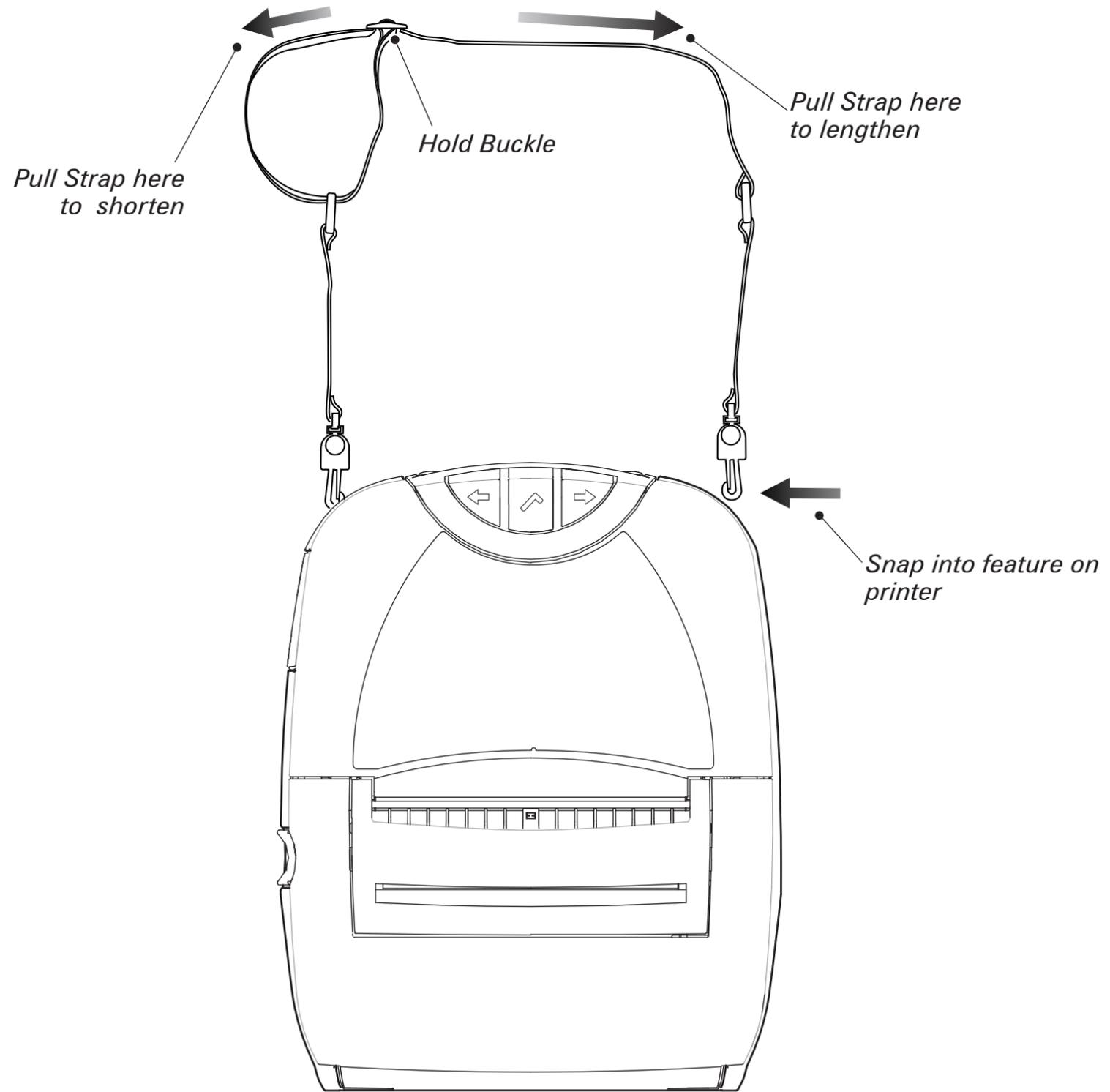
Refer to figure above. Snap each end of the shoulder strap into the retaining features on top of the printer. Hold the buckle and adjust the strap as shown until you achieve the desired length.
