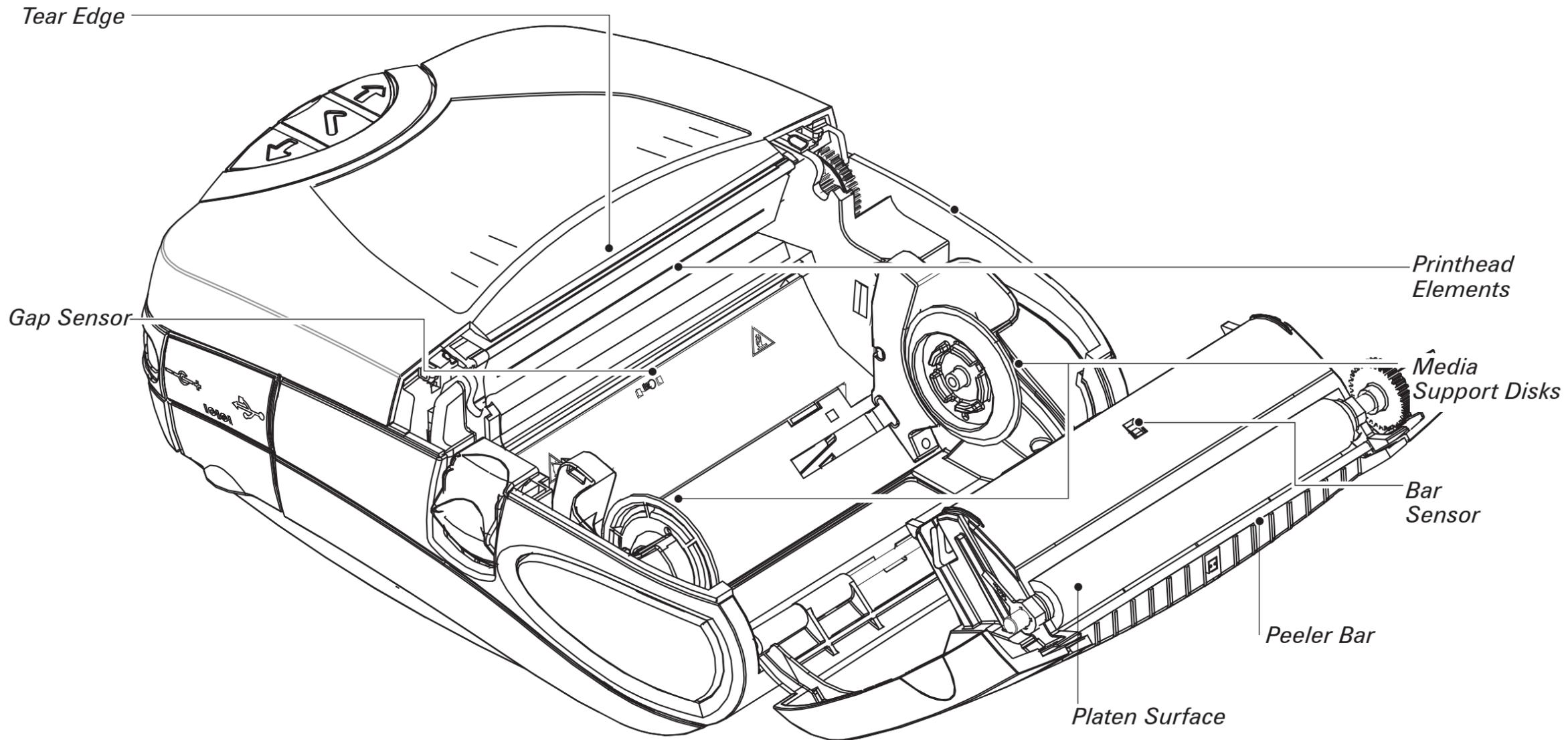
Figure 17.2- Cleaning the P4T Series Peeler Assembly
