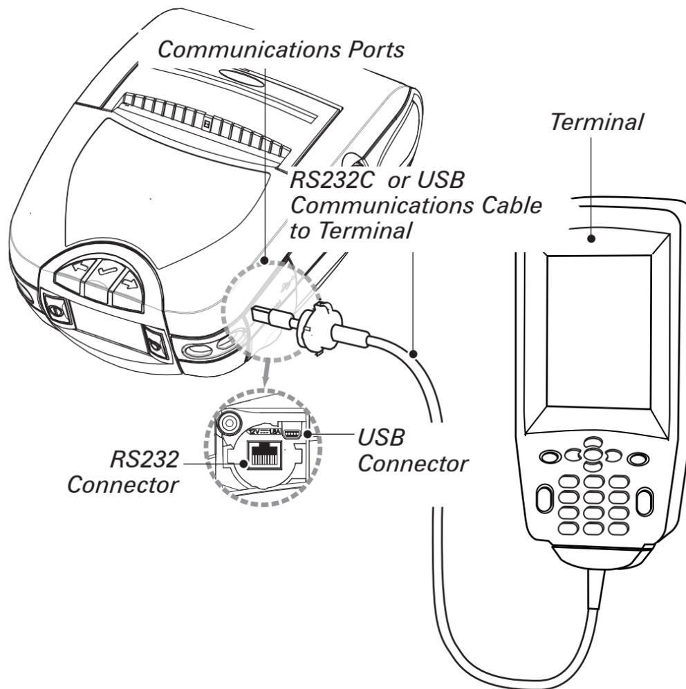
Figure 15- Connecting to a PC
