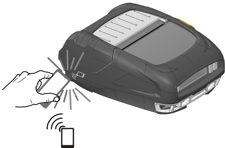
Figure 23 • Near Field Communication (NFC) Pairing
